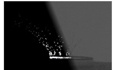
Pre-processing: Contrast enhanced and noise reduced image (left half) using the IPL compared to the original image (right half)
