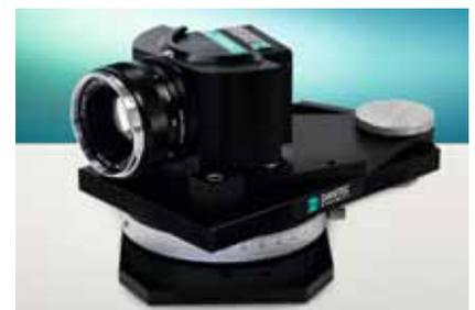
FlowSense EO 4M - one out of five models - mounted on a Scheimpflug adapter
