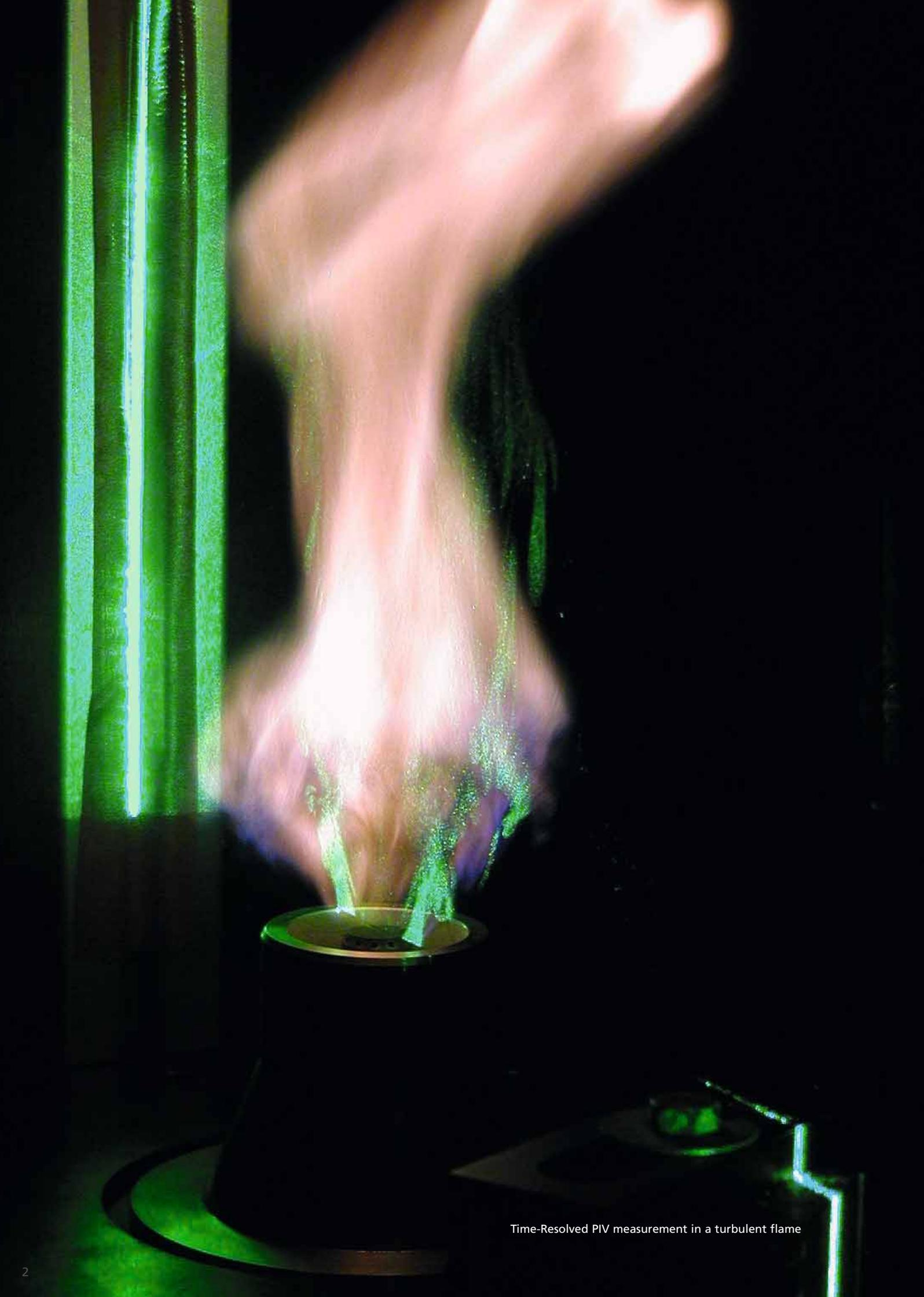
Time-Resolved PIV measurement in a turbulent flame
