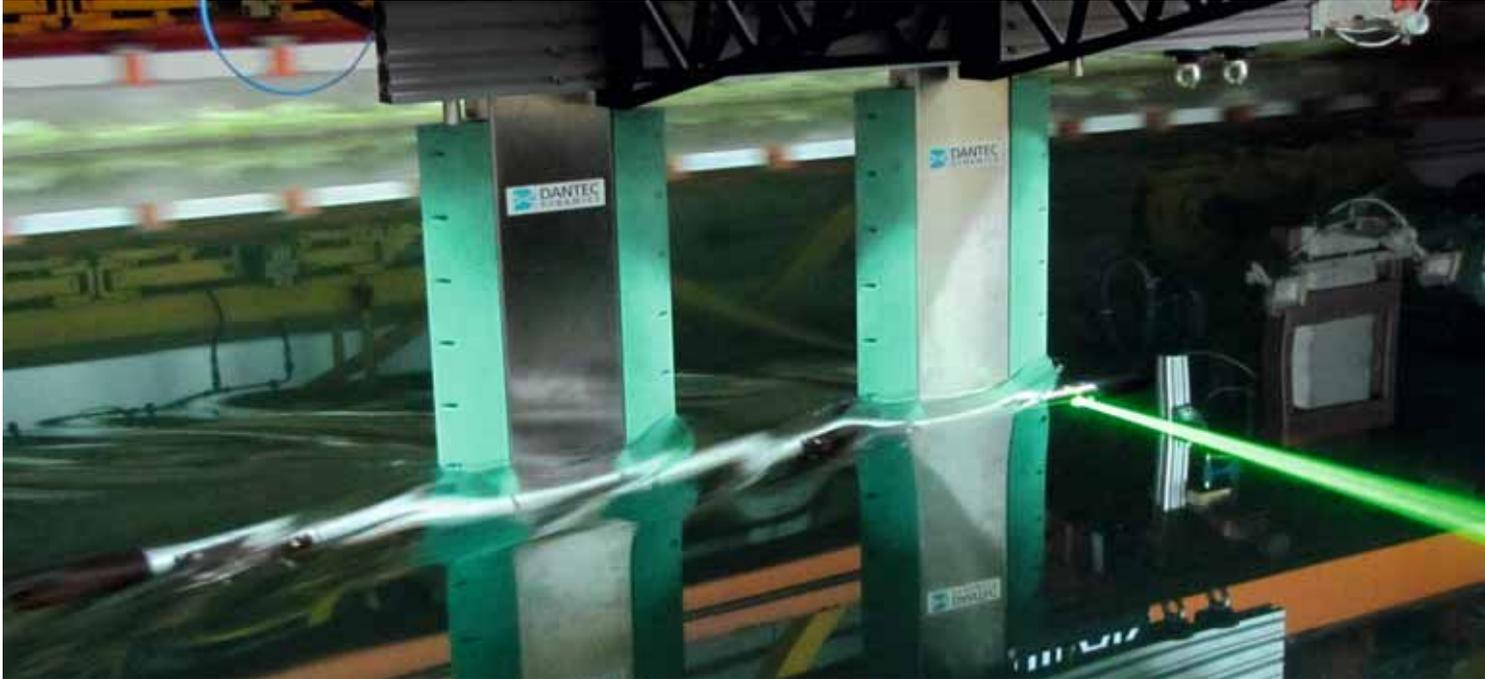
Customized Stereoscopic underwater PIV systems for towing tanks. Courtesy of CEHPAR, Spain
