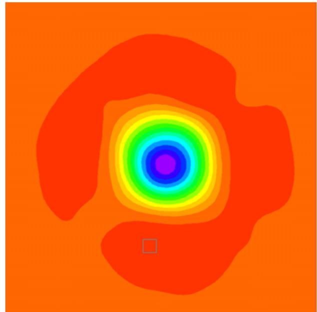
Left: Velocity field inside of a vortex calculated with 2D LSM. Right: Lambda2 vorticity criterion computed with the estimated flow gradients.
