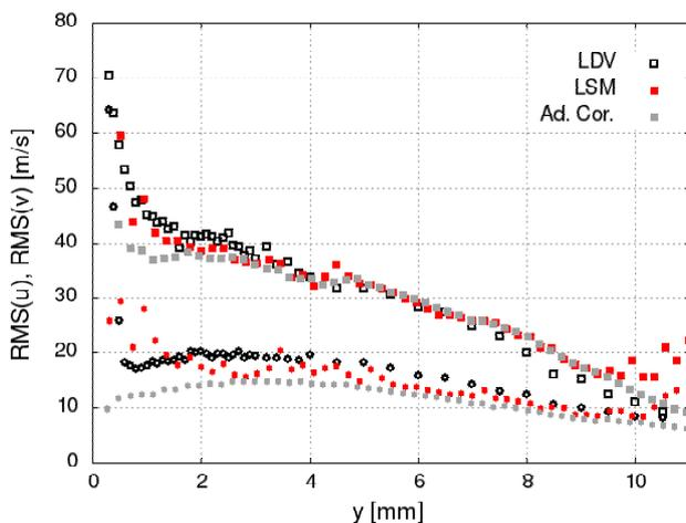
Comparison of turbulent velocity profiles from LDA and PIV. PIV interrogation window 64x32 pixels. (Courtesy of the Supersonic Group of the IUSTI, Marseille).
