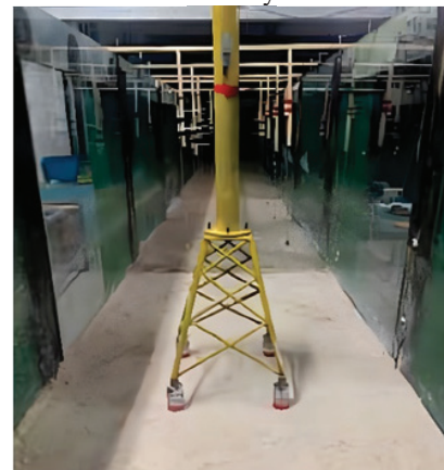
Figure 2. The jacket foundation model
