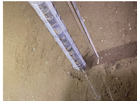
Figure 1. scour hole around the cylinder
