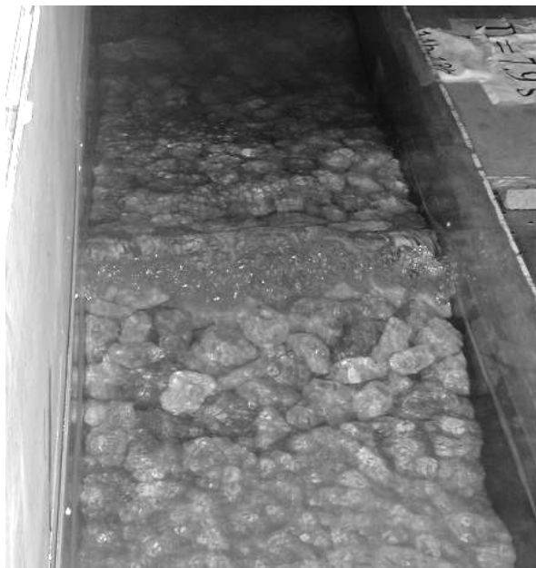
Figure 2. Pictures of the rubble mound structure taken during one of the experiments.
