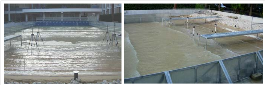
Figure 3. Pictures taken during tests. Two couples of wave gauges are visible at leading side and trailing side of the submerged barrier.
