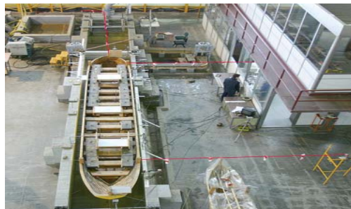
Figure 5. Mechanical system for reproducing wind (cables in red)
