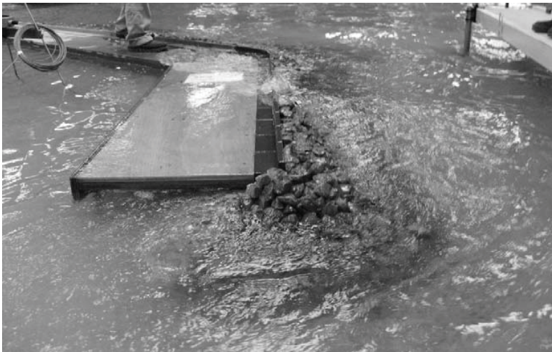
Figure 4. Snapshot of an overtopping event on the extended breakwater (during a one in 10-year wave test)
