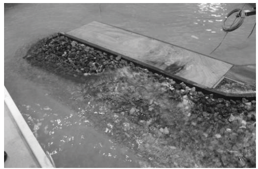
Figure 3. Wave attack on the Smith Embankment extension
