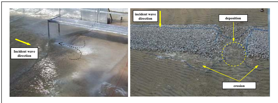
Figure 4. Current pattern and sediment processes at the gap of the barrier.
