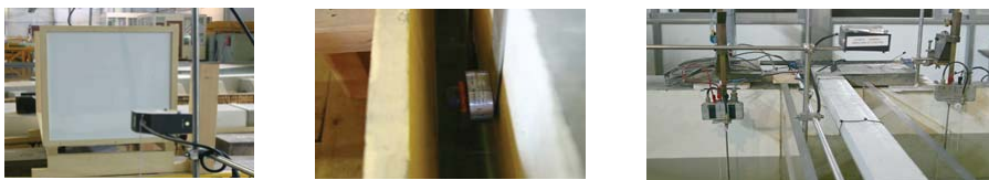
Figure 6. Monitoring. Details. Sensor laser, strength cellule (fender) and electric level gauge.
