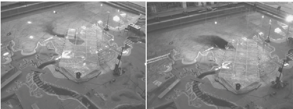
Figure 2b - Plume effluent discharge ( Q = 3.34 \text{ m}^3/\text{s} ) from Santos outfall with 4 km length (left) and 5 km length (right) after 6 tide cycles.
