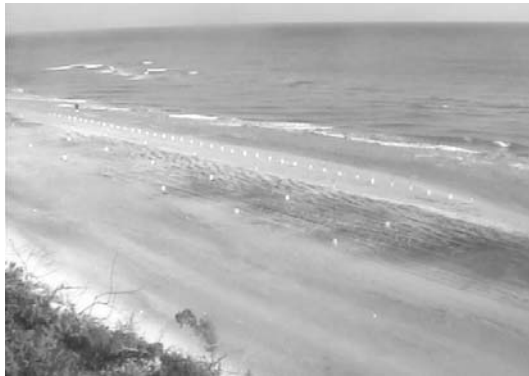
Figure 1. Alimini beach during topographic survey; vertexes of materialized grid are visible.
