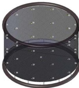
Fig. 2: The placing and numbering of LED markers on the net cage
