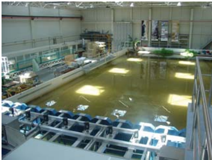
Figure 2. Wave tank of the Hydraulics Laboratory of the Faculty of Engineering of the University of Porto and barriers scheme.
