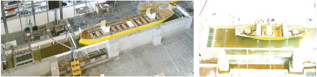
Figure 3. Lock overview model with two vessels (Bulk carrier and LPG tanker)
