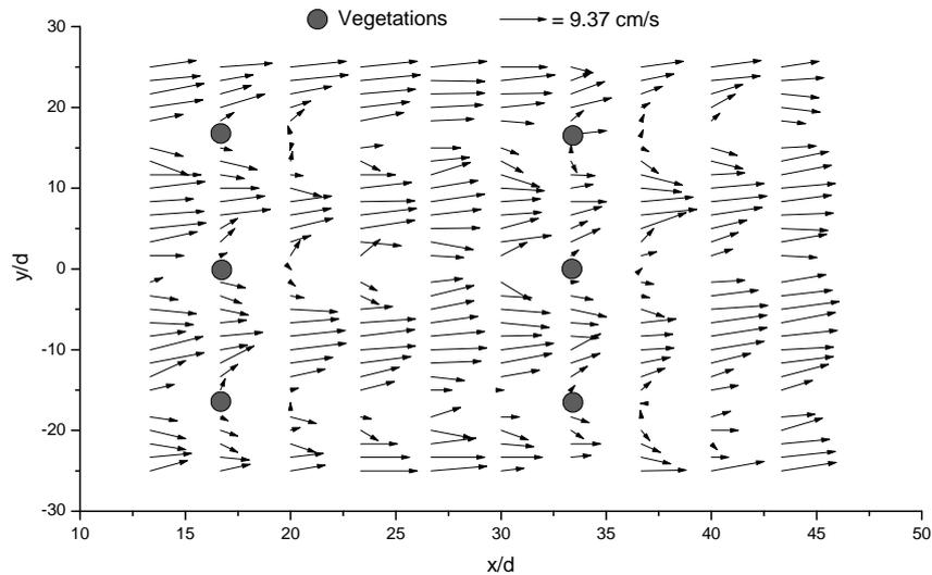
**Figure 2.** Vegetation effects on the flow velocity distribution in the horizontal plane ( $x$ - $y$ ), CV1.
