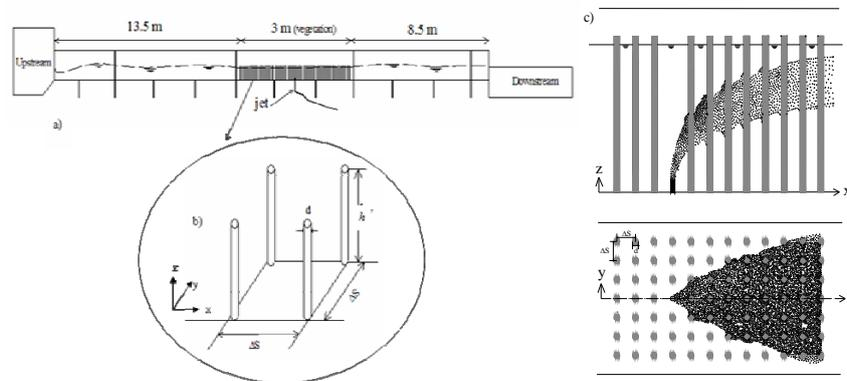
**Figure 1.** Definition sketch of: a) Channel with the vegetation canopy; b) Vegetation distribution; c) Jet diffusion within the vegetation canopies.
