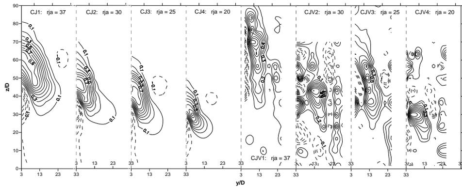
**Figure 5.** Normalized vorticity ( $\omega_x/\omega_{x,m}$ ) contours in the cross-sectional planes of  $x/D = 26.67$  for the jet discharged in both the smooth and vegetated channel.
