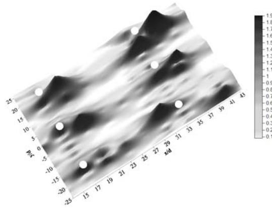
**Figure 3.** Turbulence intensity,  $rms(u')/|U|$ , distribution in the horizontal plane, CV1, white discs represent the vegetation stems.
