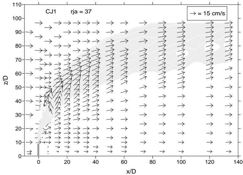
**Figure 4.** Velocity distribution in the plane of flow symmetry ( $x$ - $z$ ), CJ1.
