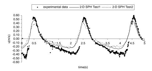
Figure 4b. Comparison of experimental and numerical horizontal velocity components (section 49, 0.1 m from the bottom).
