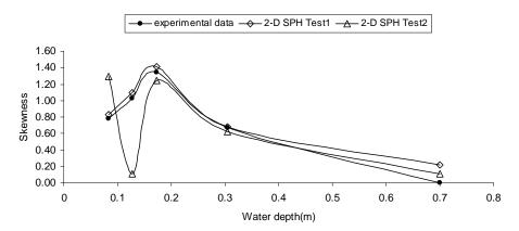
Figure 6. Comparison of experimental and numerical skewness of surface wave elevations.
