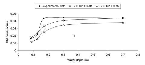
Figure 5. Comparison of experimental and numerical standard deviation of surface wave elevations.
