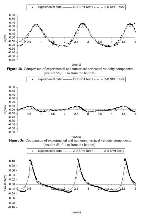
Figure 4a. Comparison of experimental and numerical wave surface elevation (section 49).
