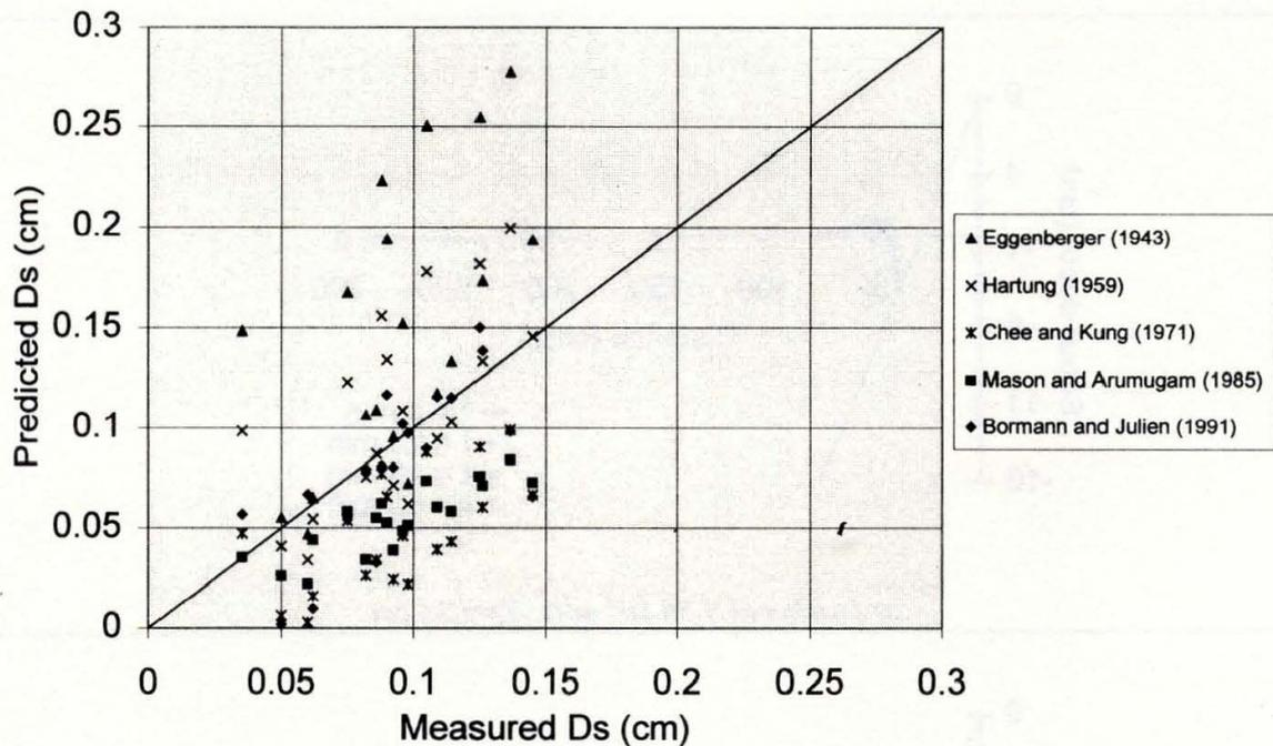
Fig. 7. Comparison of measured and calculated maximum scour depths  $D_s$ .
