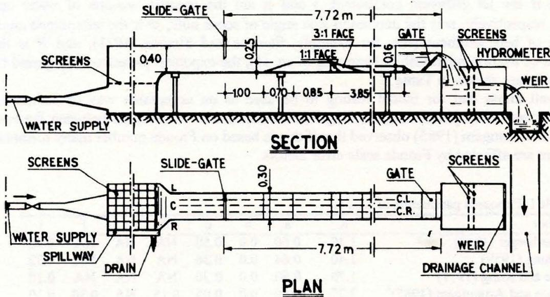
Fig. 1. Schematic view of experimental arrangement
