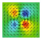
Velocity field of a vortex and dv/dx directly computed by 2D LSM
