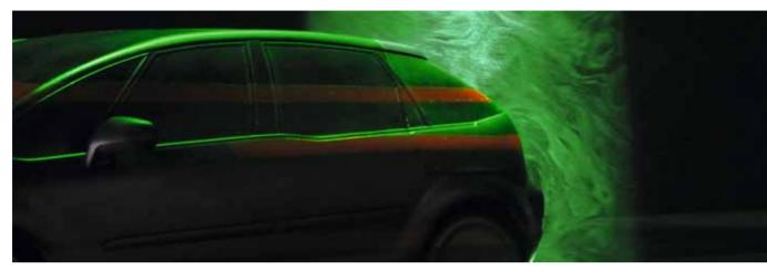
Time-Resolved PIV measurement of wake flow behind a car. Courtesy of PSA, France
