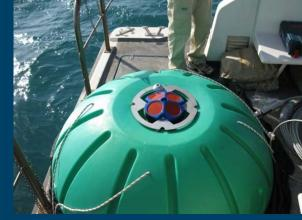
System in the Mar Grande Taranto (Italy) for the monitoring of sea currents (ADCP) and waves. Also a meteo station, a CTD, a combined fluorometers, turbidity meters and a C3 Submersible Fluorometer for CDOM, Crude Oil and Refined Fuels have been installed.
