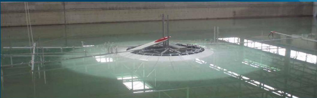
National Interest Research Program approved with D.M. N. 174/2004. TSUNAMI WAVES GENERATED BY LANDSLIDES IN WATER: MECHANICS OF WAVE GENERATION AND PROPAGATION, DEVELOPMENT OF FORECASTING TOOLS AND REAL-TIME WARNING SYSTEMS BASED ON TIDAL MEASUREMENTS. The photo shows a tsunami scenario generated by landslide at Sciarra del Fuoco (Stromboli island). The physical model was constructed at the LIC of the Technical University of Bari.
