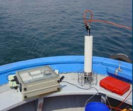
Sea current measurements: **VM-ADCP** with GPS receiver (the accuracy of the GPS velocity should be 0.05 m/s or better (DGPS) Gyro: with serial output and accuracy better than 1°. It is also possible to use combined gyro and GPS system <u>Computer: The survey</u> computer needs at least 3 serial ports and it is advisable to use an
