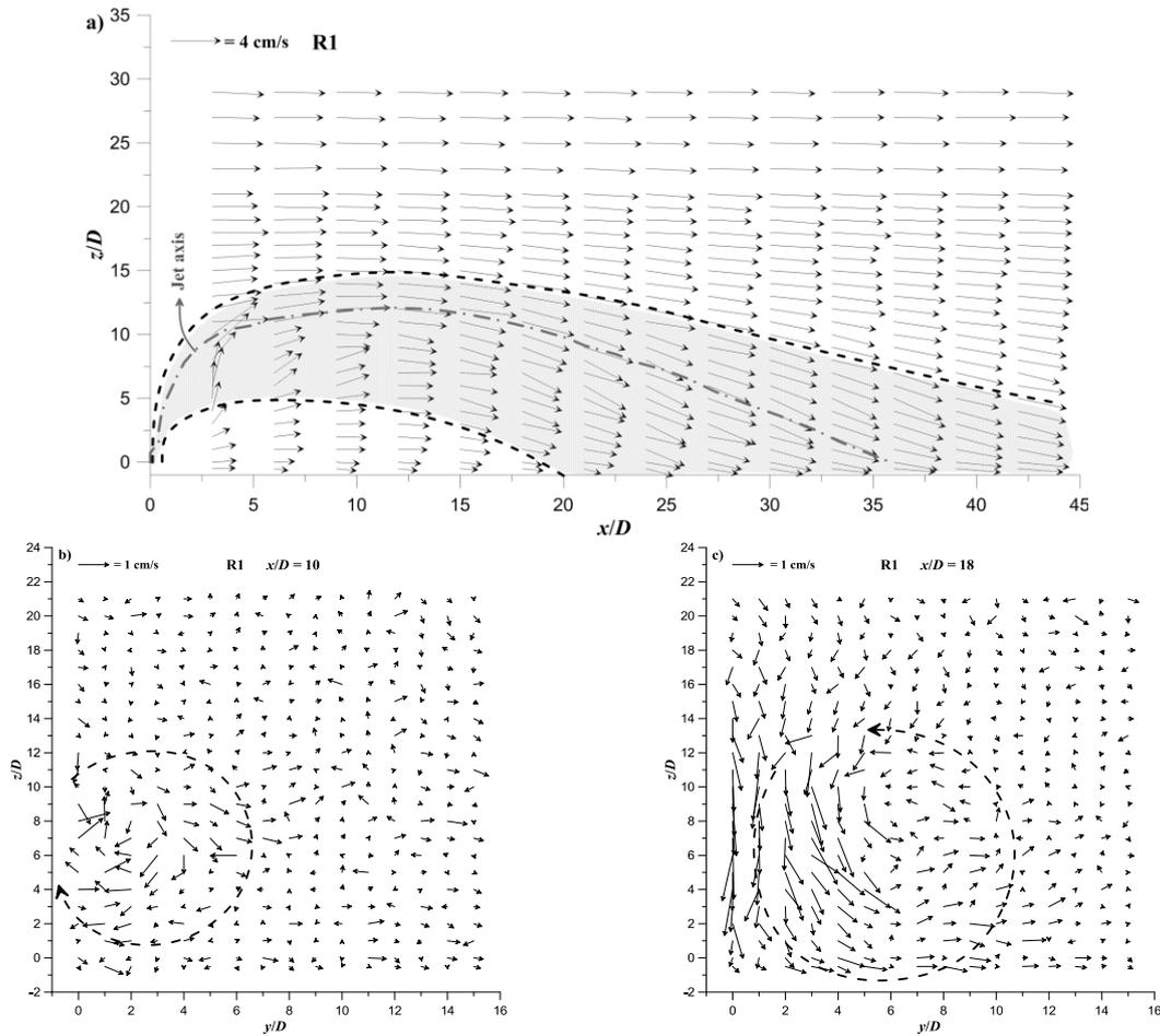
**Figure 2.** Velocity flow-field of run R1, as an example: a) jet penetration in the  $(x, z)$ -plane of flow symmetry ( $y=0$ ), where  $y$  is the transversal direction, b) CRVP in the cross-section at  $x/D=10$ , ascending region, c) CRVP in the cross-section at  $x/D=18$ , descending region.
