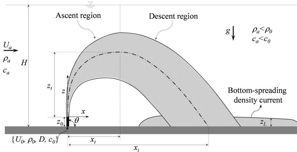
**Figure 1.** Definition sketch of the vertical dense jet in shallow water, where  $g$  is the gravity acceleration,  $(x, y)$  are the longitudinal and vertical coordinates, respectively, and  $z_L$  is the thickness of the bottom-spreading layer of the density current.
