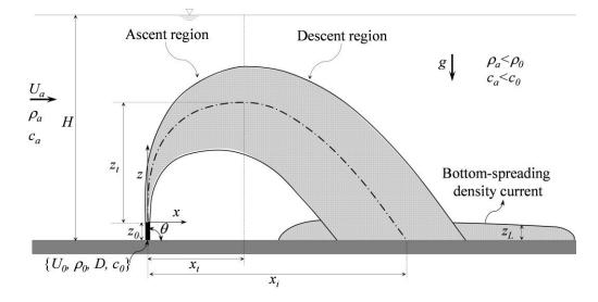
**Figure 1.** Definition sketch of the vertical dense jet in shallow water, where g is the gravity acceleration, (x, y) are the longitudinal and vertical coordinates, respectively, and  $z_L$  is the thickness of the bottom-spreading layer of the density current.
