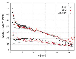
Comparison of turbulent velocity profiles form LDA and PIV. PIV interrogation window 64x32 pixels. (Courtesy of the Supersonic Group of the IUSTI, Marseille).
