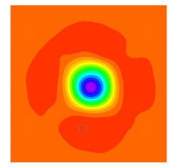
Left: Velocity field inside of a vortex calculated with 2D LSM. Right: Lambda2 vorticity criterion computed with the estimated flow gradients.
