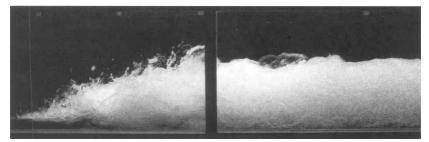
Fig. 1. A typical hydraulic jump with inflow Froude number equal to 5 (by Hager, 1990).
