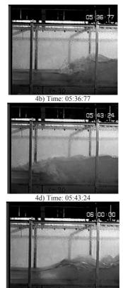
4e) Time: 05:55:93 Fig. 4. Typical oscillatory flow patterns between B-jump and Wave jump; time is expressed in minutes, seconds and hundredths of seconds from the shooting start.
