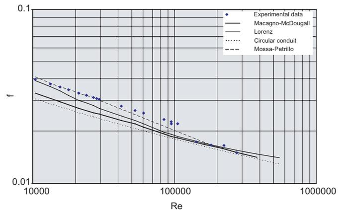
Figure 10 Resistance coefficients against Reynolds number.
