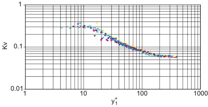
Figure 4 Turbulence index against  $y_1^+$ .
