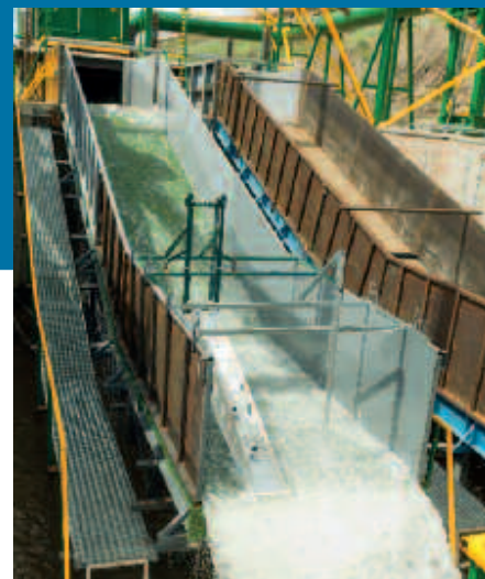
Figure 3 - Wave-overtopping of a grassed, soil slope placed in the wave-overtopping facility
