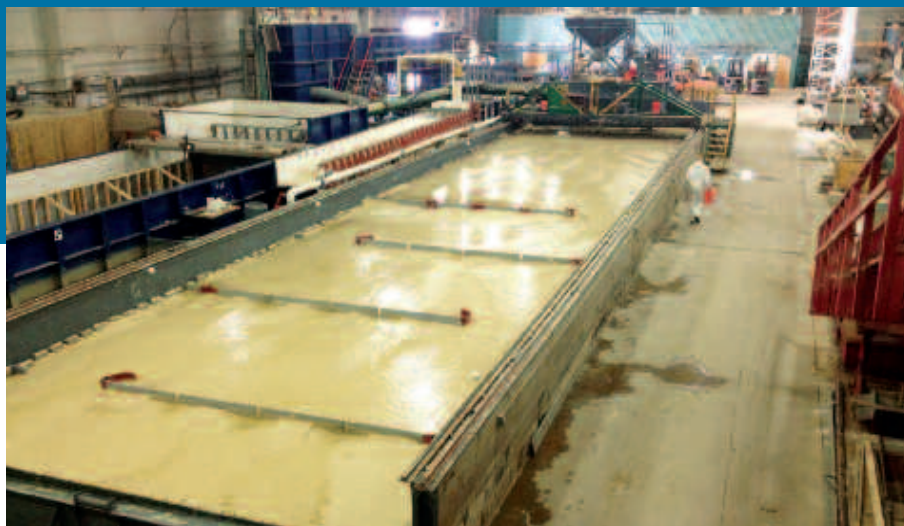
Figure 2 - The 8 m by 33 m flume used to model a system of grade-building structures placed in a mobile-bed model of a braided alluvial channel
