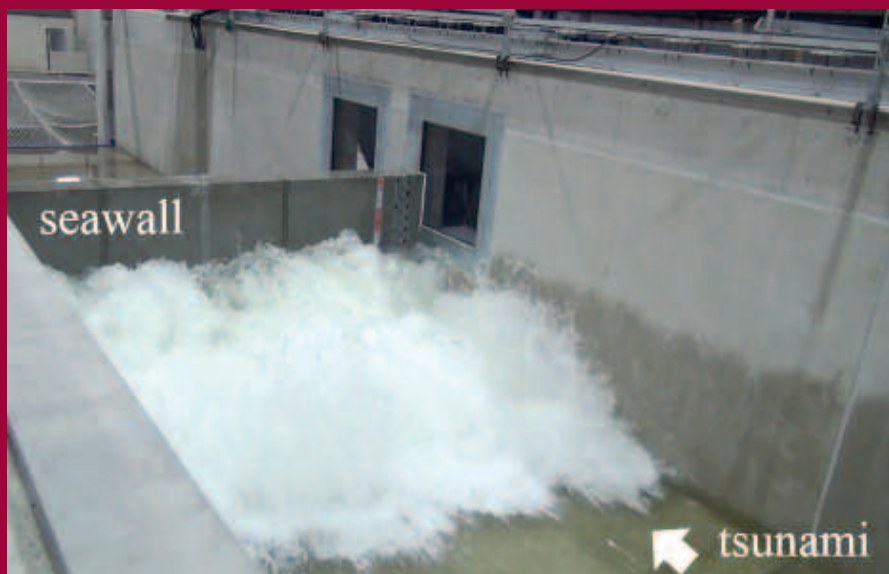
Figure 3 The experiment on tsunami wave pressure loading on a seawall
