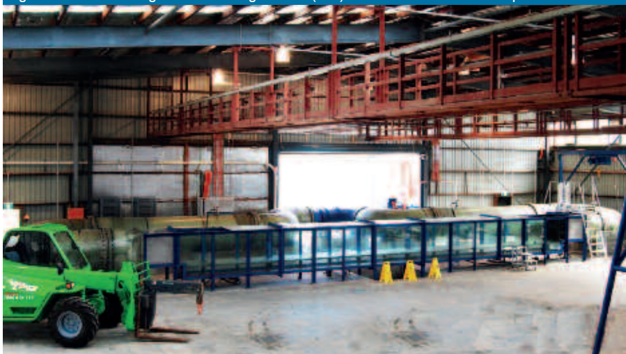
Figure 2 - General arrangement of the large O-tube (LOT) at UWA's Shenton Park campus
