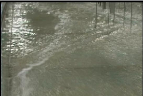
A close-up photograph of the hydraulic jump, showing lateral shock waves and a circulation zone. The water is highly turbulent and frothy.  |
