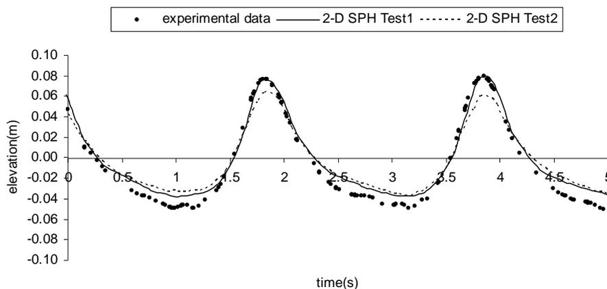
**Figure 3a.** Comparison of experimental and numerical wave surface elevation (section 55).
