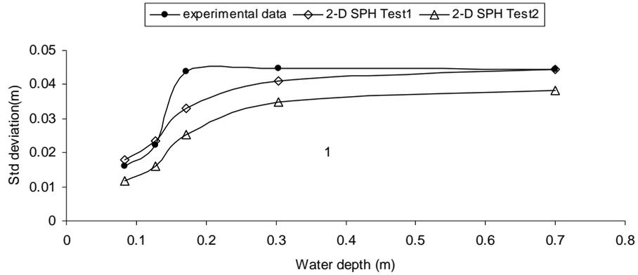
**Figure 5.** Comparison of experimental and numerical standard deviation of surface wave elevations.
