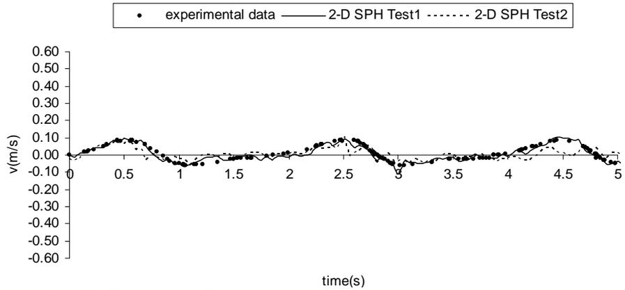
**Figure 3c.** Comparison of experimental and numerical vertical velocity components (section 55, 0.1 m from the bottom).
