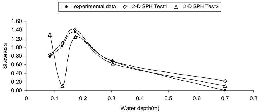
**Figure 6.** Comparison of experimental and numerical skewness of surface wave elevations.
