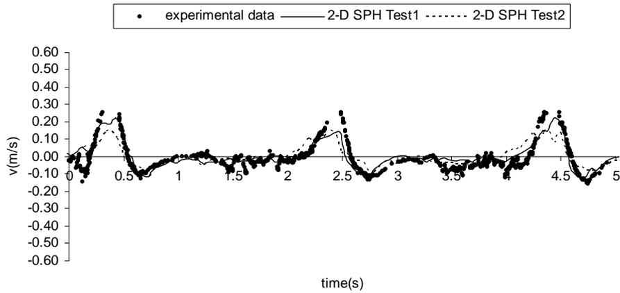
**Figure 4c.** Comparison of experimental and numerical vertical velocity components (section 49, 0.1 m from the bottom).
