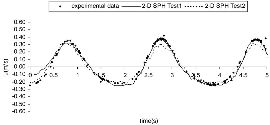
**Figure 3b.** Comparison of experimental and numerical horizontal velocity components (section 55, 0.1 m from the bottom).
