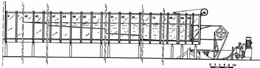
Figure 1. Sketch of the wave flume.
