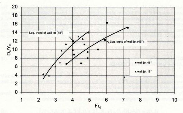
Fig. 8. Ratio of the measured scour depths and  $Y_0$  versus  $Fr_d$
