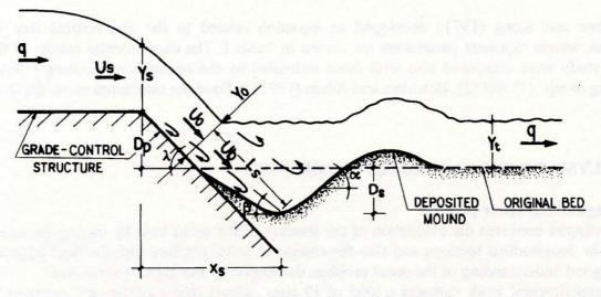
Fig. 2. Definition sketch of the jet path
