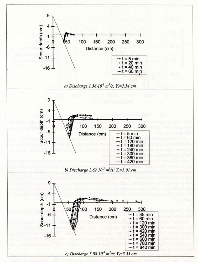
Fig. 6. Variation of scour profiles with time ( $\lambda = 18^{\circ}$ )
