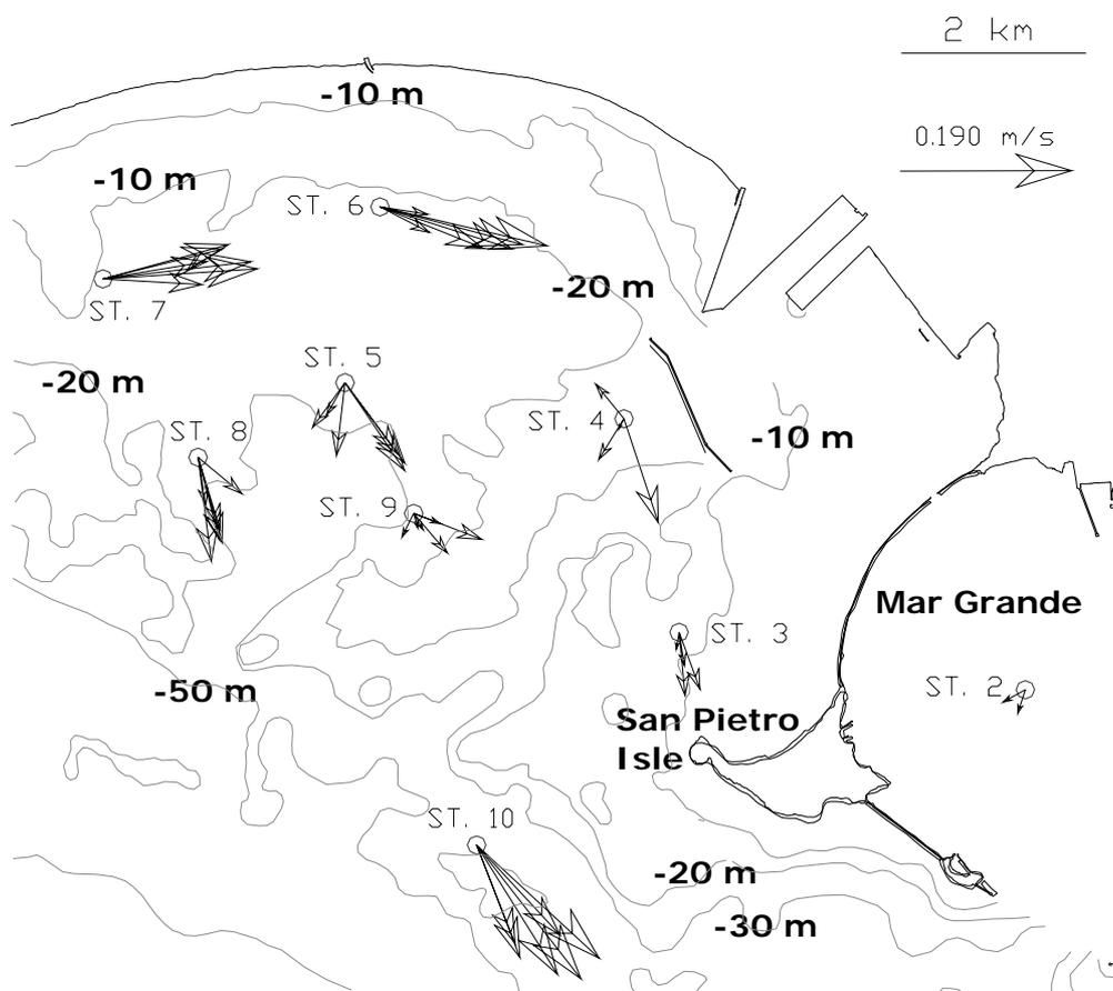
Figure 3. Stationing point displacements and measured mean velocities at selected depths
