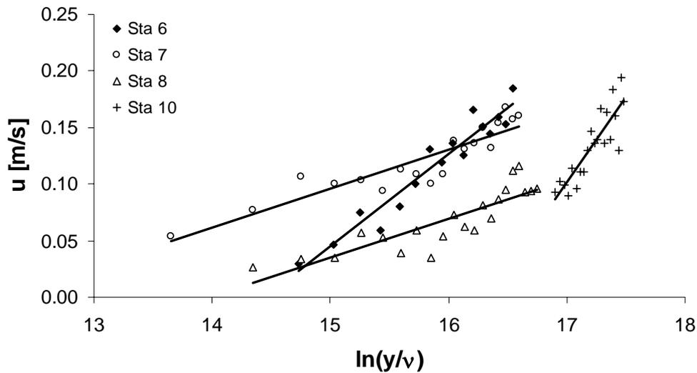
Figure 7. Fitting straight lines used to obtain the shear velocities at the investigated stations
