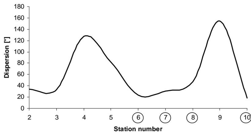
Figure 5. Maximum dispersion of the velocity direction at each station and along the depth (the circled stations were considered for logarithmic plots)
