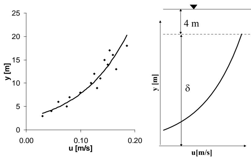
Figure 6. Typical logarithmic velocity profile (station 6)
