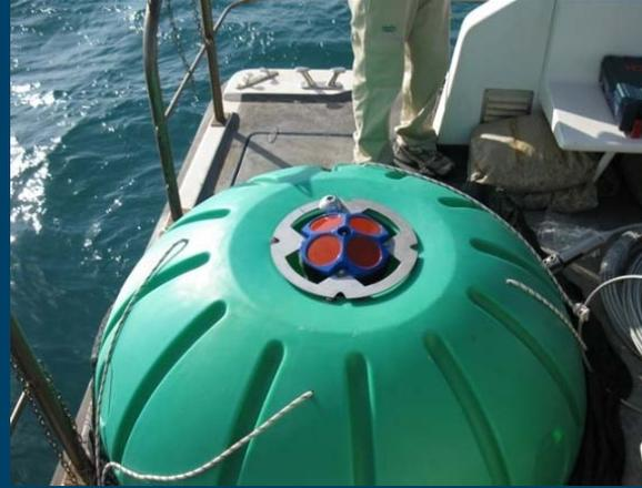
System in the Mar Grande Taranto (Italy) for the monitoring of sea currents (ADCP) and waves. Also a meteo station, a CTD, a combined fluorimeters, turbidity meters and a C3 Submersible Fluorometer for CDOM, Crude Oil and Refined Fuels have been installed.
